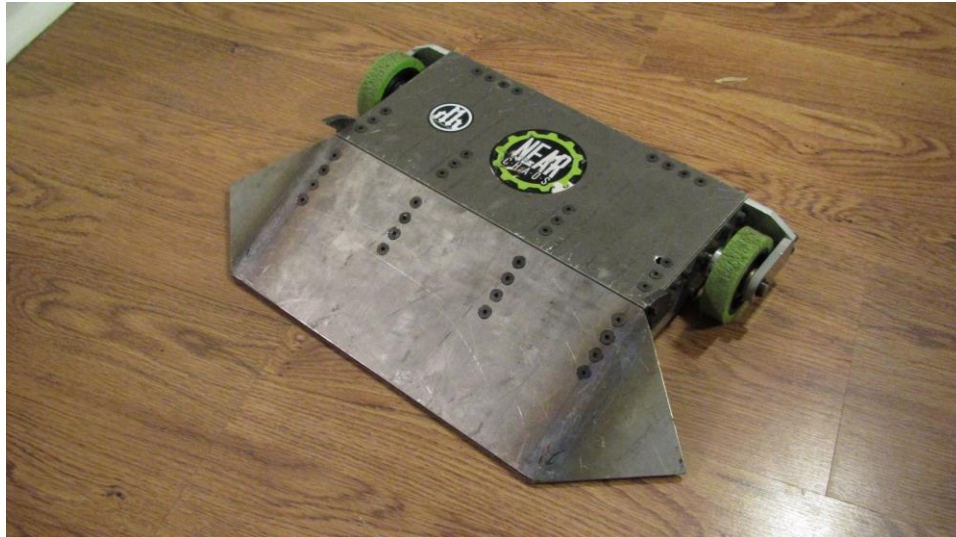
Shaped titanium wedge, magnesium top plate and 6061 frame all fabricated by Team Whyachi
