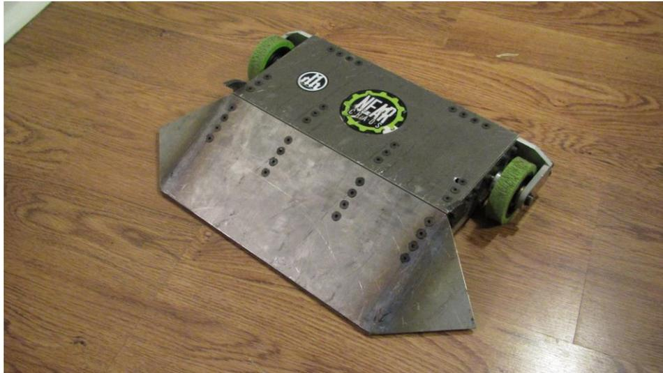
*Shaped titanium wedge, magnesium top plate and 6061 frame all fabricated by Team Whyachi*
