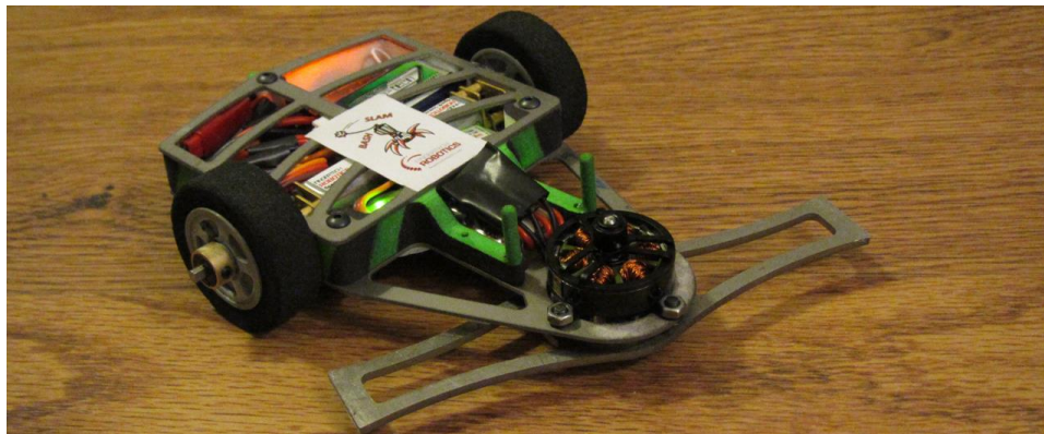
150g Robot with printed sintered Nylon chassis from Shapeways
